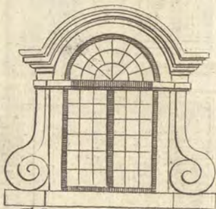
A Lantern with a Semi- circular Arch.
